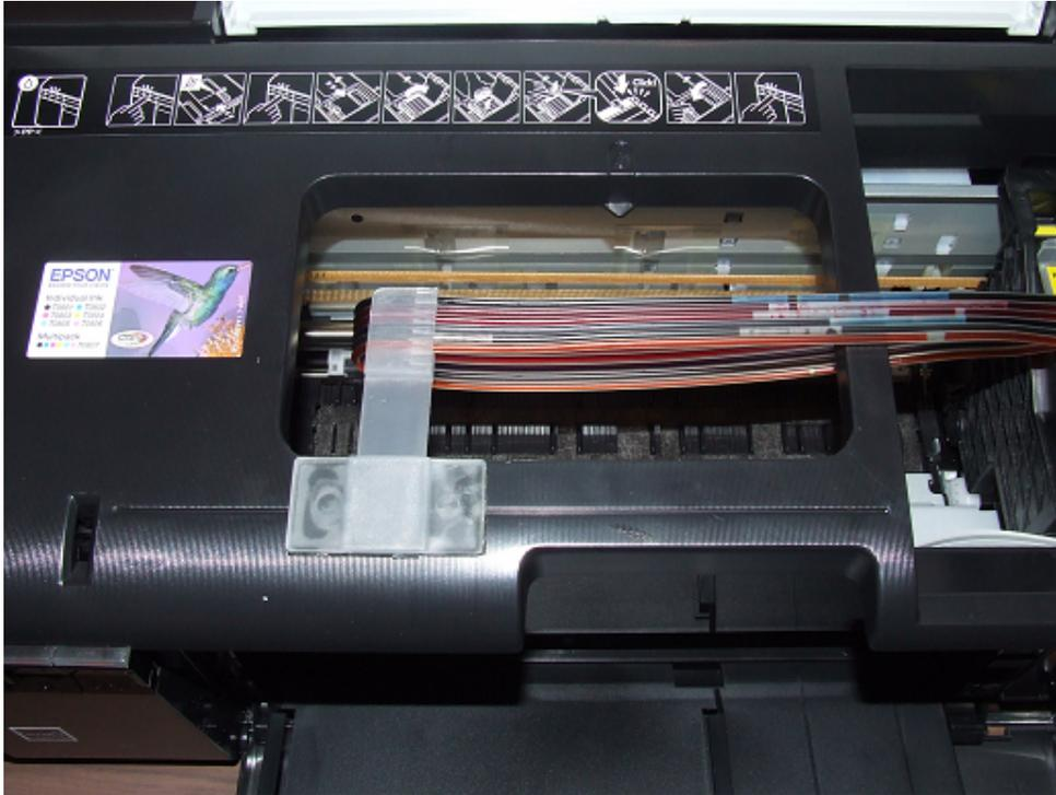
Keep the piping straight and now clip into the small clip on the side, as shown below.
