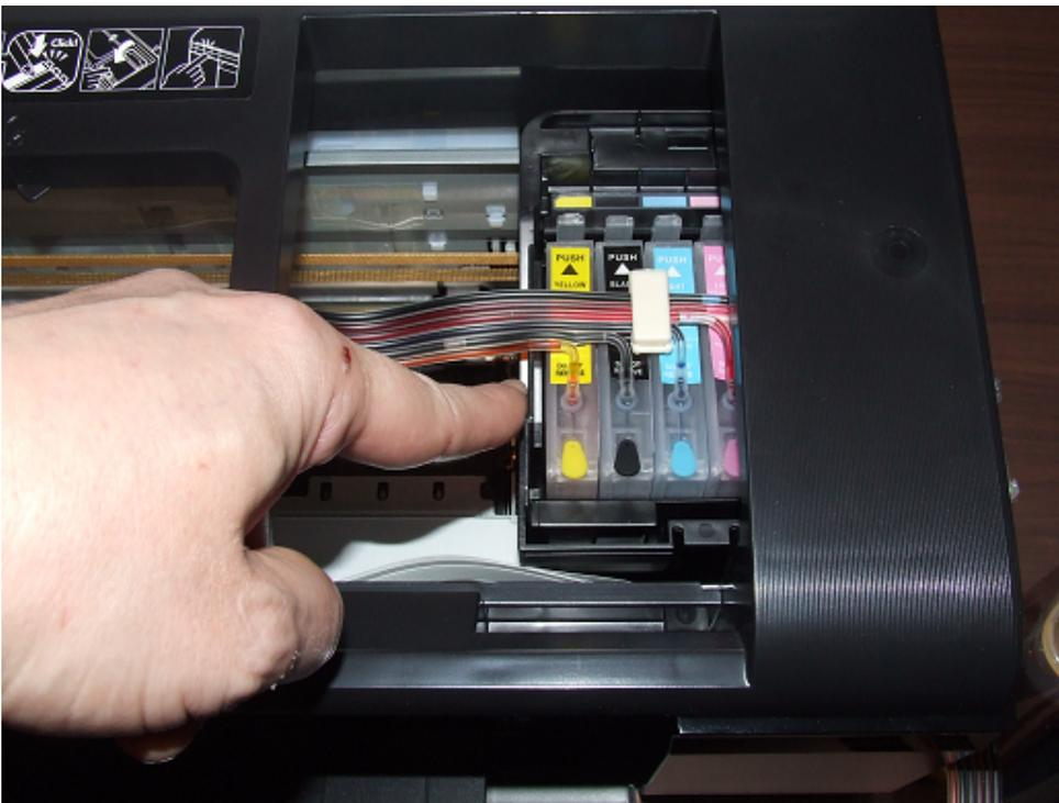
Now you can put the piping into the long clip that you fixed to the printer earlier. Make sure that there is an inch or two give in the bottom stretch of the piping, this allows for the movement of the carriage. Put the piping exactly as below:
