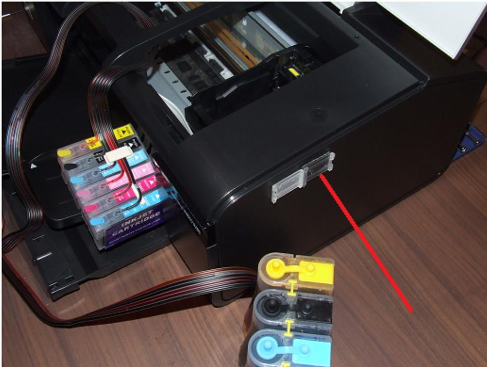
Next step is to stick the long plastic holder to the printer as shown below:
