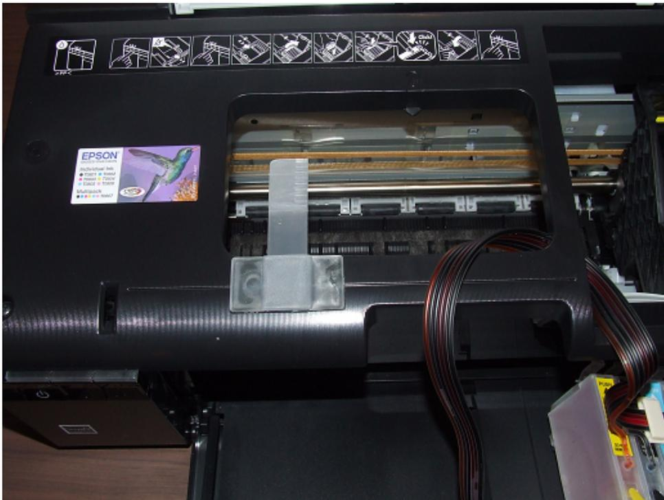
Now place the cartridge block into the carrier and make sure you click each cartridge down, they MUST click in. Make sure they click in in at a time, as shown below:
